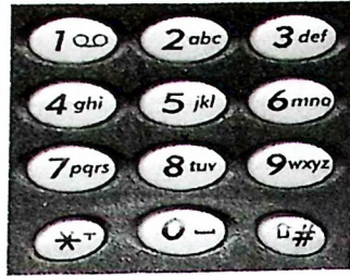
Fig. 1. A mobile phone keypad following the ITU-T E.161 mapping of numeric keys to alphabetic symbols. Non-standard mappings exist for key 1 (symbols such as punctuation), key 0 (spaces), and the * and # keys – one of which is usually assigned to “cycle”
